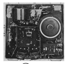
The Model 501 Model 501 Rapid Scanning Spectrometer Scans 30A/usec. with Excellent Stability & Resolution; Covers Broad Wavelength Region in One Scan.
