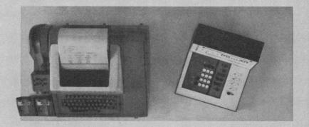
Name familiar but you can't remember the face? The insides of this new Mathatron computer calculator are different, too. Log, antilog, sine, cosine, and arctan are performed at the touch of a button. Storage 4000 bits. Simplified program control. And the price-performance ratio is higher than any other computer/ calculator. Starts at \$6990.
