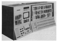
THE 505 CAN EXPAND TO 186 AMPLIFIERS, COMPARED TO 80 MAXIMUM FOR ITS LEADING COMPETITOR.
