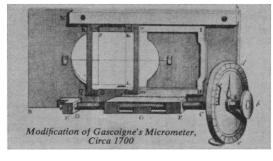
Three hundred and twentyseven years ago, William Gascoigne of Yorkshire constructed a micrometer measuring device suitable for use in the relatively crude optical instruments of that day. Since 1639 many refinements have been made upon
