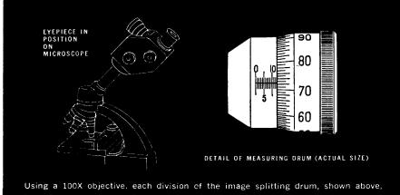
is equivalent to a dimension on the microscope object of 0.084  $\!\mu$  (0.000003 inches.)
