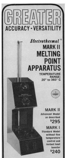
OPERATION: Uses established technique of melting samples at the bottom of vertical capillary tubes. Up to three samples are placed in the shielded low heat capacity metal block, illuminated and viewed through a deep fixed focus lens.
