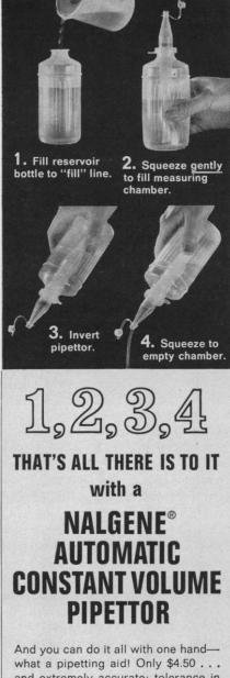
and extremely accurate: tolerance in ml is  $\pm$  .02, .02, .04 and .06 for the 1, 2, 3 and 5 ml sizes, respectively. Use several for procedures requir-
