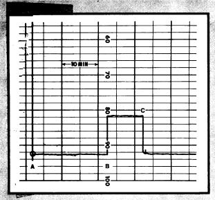
Model 303 double-beam system eliminates the effects of drift in lamp, detector, and electronics. Here, Ca is run from a cold start. Burner is lighted at A, 1 ppm Ca inserted at B, withdrawn at C. Quiet, stable baseline commonly produces 5X improvement in detection limit and precision.
