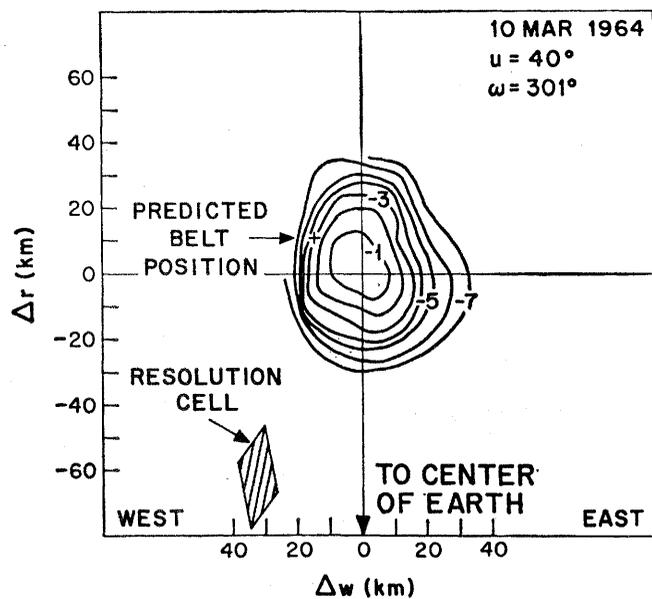
Fig. 2 (left). Physical cross section of the dipole belt at apogee. Contours of equal dipole density are labeled in decibels referred to the density at the origin. The angle  $u$  denotes the argument of latitude of the observation whereas  $\omega$  denotes the argument of perigee. Fig. 3 (above). Same as Fig. 2, except here the observed section was near a semilatus rectum point of the orbit.
