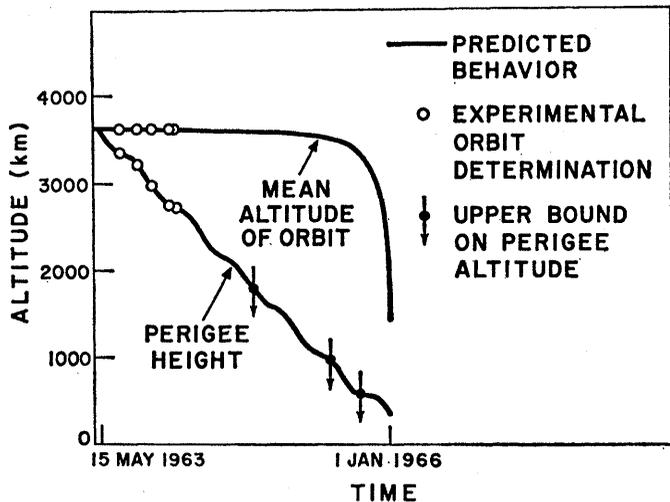
Fig. 4 (above). Orbital behavior of the West Ford dipole belt: comparison between theory and observation.
