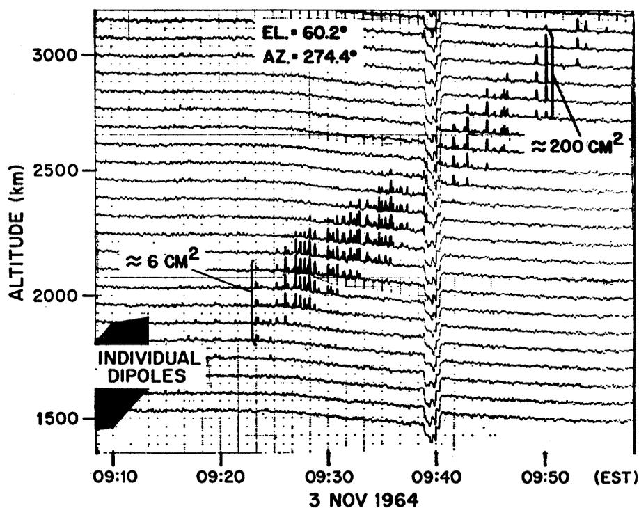
Fig. 1. Millstone Hill radar observations of dipole clusters at 1295 Mcps.
