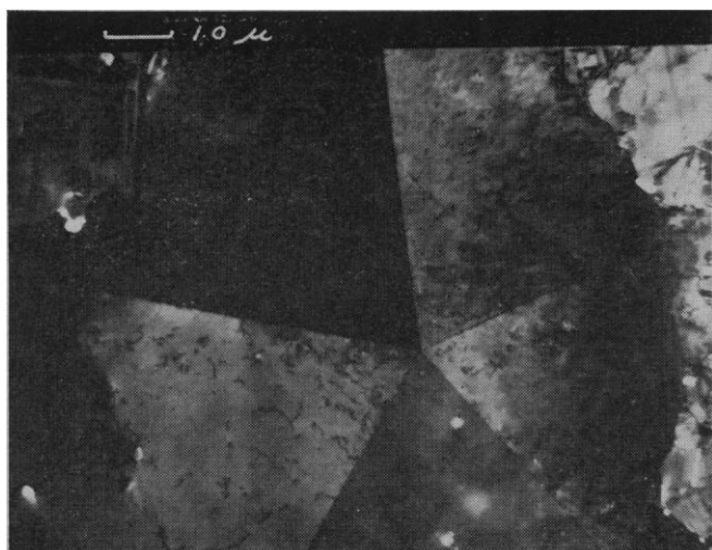
Fig. 2 (left). Transmission electron micrograph of a pseudo-fivefold nickel grain oriented normal to the foil. Fig. 3 (right). Electron micrograph showing both tilted and nontilted pseudo-fivefold grains.
