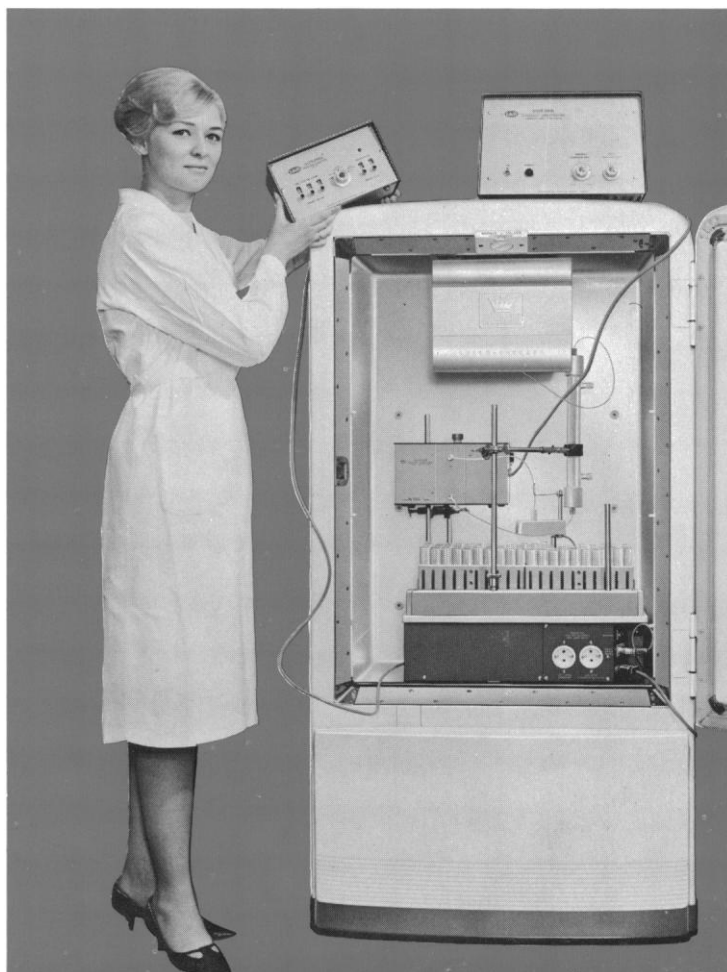
The UltroRac, complete with separation column, ready for operation in a normal domestic refrigerator
