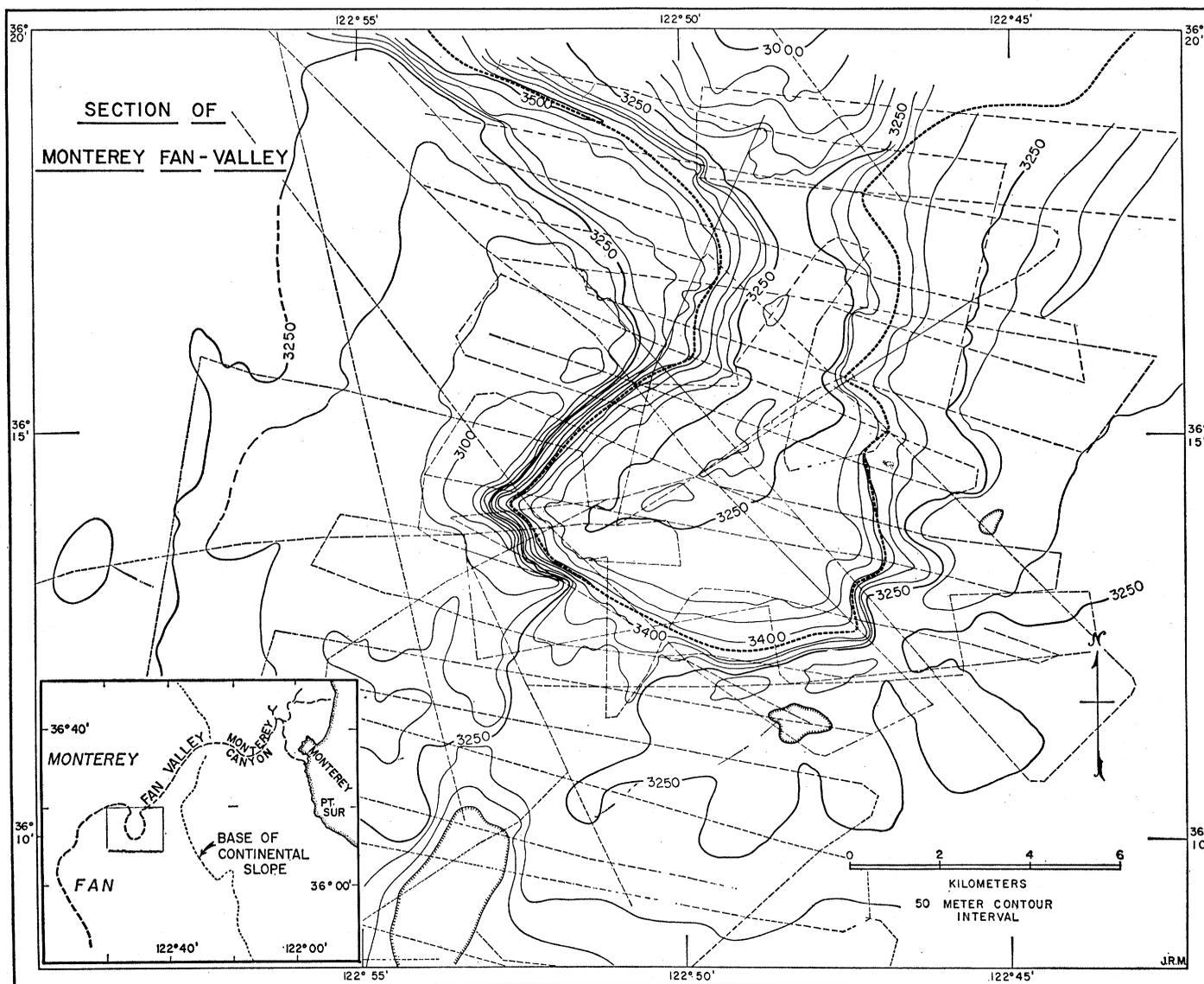
Fig. 1. Contours of a large meander in the valley crossing the submarine fan seaward of Monterey Canyon. Relation to Monterey Canyon and the coast at Monterey are given in the inset along with approximate base of continental slope and Monterey seafan. Long dashed lines indicate locations of closely spaced sounding network on which the contours were based. Heavy short dashed line shows valley axis. Relative locations were obtained by radar ranges and bearings on a centrally located buoy.
