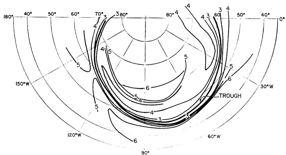
Fig. 6. A contour map, drawn from Alouette I observations on successive orbits, which shows a deep electron-density trough at high latitudes. The extraordinary penetration frequencies (in megacycles per second) shown here indicate nearly an order-of-magnitude density decrease at the peak of the ionosphere. [Adapted from the work of D. B. Muldrew (22)]
