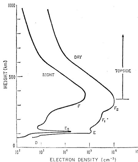
Fig. 1. Vertical profiles of the electron density in the typical ionosphere. The topside sounders measure the ionospheric properties above the altitude of maximum density (that is, in the "topside").
