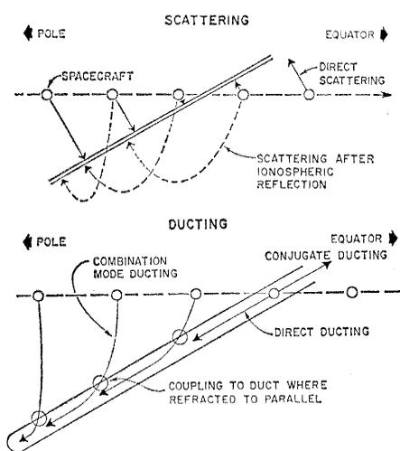
Fig. 5. The geometry of echoes from electron-density irregularities observed by the topside satellites. Thin irregularities scatter the radio energy. Thick irregularities duct the radio energy along the magnetic field—even to the conjugate reflection point in the opposite hemisphere.
