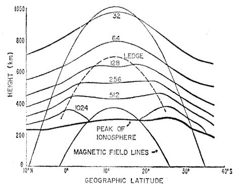
Fig. 4. A topside-sounder observation of the equatorial anomaly over South America, 1550 local time, 17 February 1963. The distribution of electron density in the anomaly is controlled by the earth's magnetic field. (Unit of electron density:  $10^8$   $\text{cm}^{-3}$ .)
