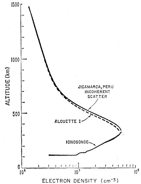
Fig. 3. Simultaneous Alouette I and ground-based measurements of electron density over South America, about 2015 U.T., 28 May 1964. The agreement is good, except for a small discrepancy near the peak of the ionosphere.
