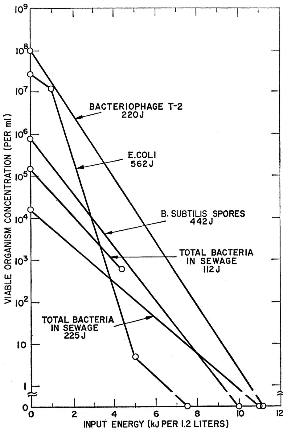
Fig. 2. Typical electrohydraulic sterilization data: viable organisms versus input energy. Numbers indicate joules per discharge.
