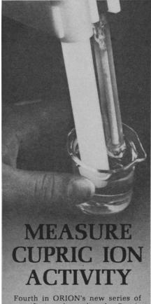
Fourth in ORION's new series of specific ion electrodes, the Cupric Ion Activity Electrode, Model 92-29, permits for the first time the direct, rapid measurement of +2 copper in aqueous solutions.
