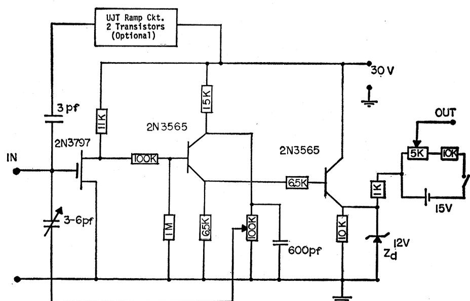
Fig. 1. Schematic diagram of the IGFET amplifier. For resistance values, K = 1 kohm. The UJT ramp circuit is used to check electrode resistance *in situ*. The 2N3565 are low-noise transistors operated at unity gain. Negative capacitance compensation is provided by the variable capacitor.
