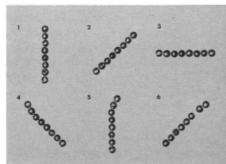
Fig. 1. A chain of eight spheres formed by applying an electric field in the vertical direction (1). With the electric field off, and the shear field on, the chain rotates clockwise (2, 3), buckles under axial compression (4, 5), and finally breaks under tension (6).
