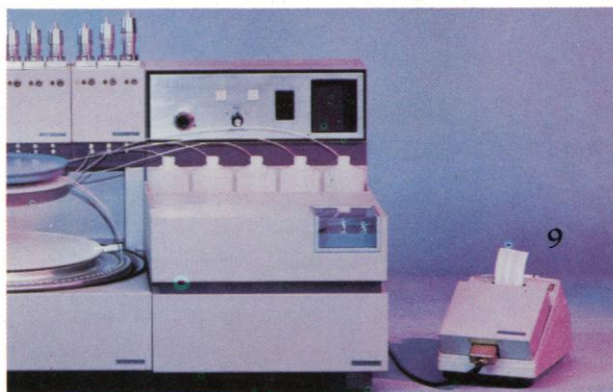
1. Master controller, 2. Rack handler, 3. Transfer probe, 4. Pipetter, 5. Reagent dispensers, 6. Process module, 7. Data converter, 8. Spectrophotometer, 9. Printer.
