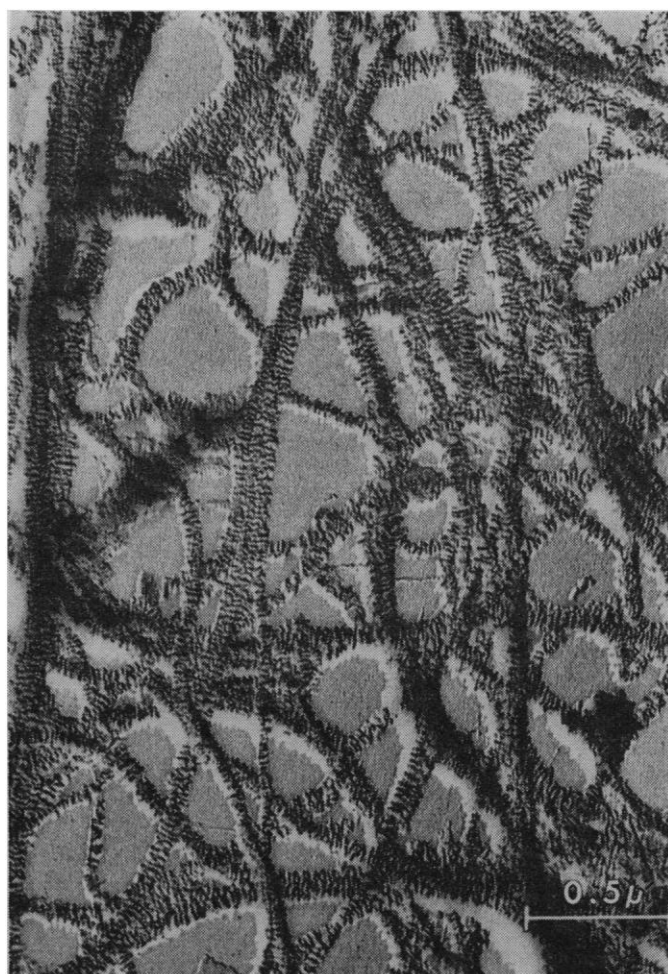
Fig. 1 (left). Photomicrographs showing (A) globules of isotactic polystyrene freed of catalyst and resuspended in toluene (crossed Nicol prisms); (B) a preparation similar to that in A with the focus adjusted to show the skin of the globules (crossed Nicol prisms); (C) a portion of a polystyrene globule which had been dried on a glass slide and replicated (electron micrograph, Pt-Pd shadow cast). Fig. 2 (above). Fibrils similar to those in Fig. 1C, obtained by mechanically disrupting a globule of isotactic polypropylene. Electron micrograph, platinum shadow cast.
