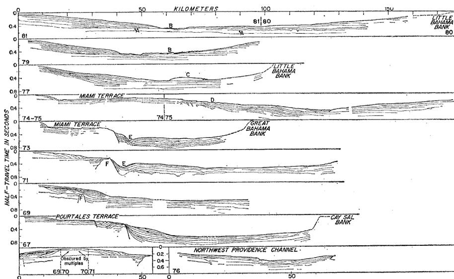
Fig. 2. Continuous seismic profiles across the Straits of Florida. The profiles have a vertical exaggeration of  $10 \times$ . Areas marked by letters A to F indicate the special features described in the text. For location of profiles see Fig. 1.
