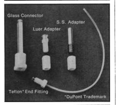
Chemically inert Zero dead volume 500 psi pressure rating For 1/16" Teflon\* tubing
