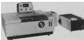
Single-beam, double-grating. UV-visible range: 190m $\mu$ -700m $\mu$ . Large sample compartment (6" x 6" x 8 $\frac{1}{16}$ "). Choice of collimating or focusing optics. Wavelength accuracy—.5A. Wavelength graduations—.2m $\mu$ . Combination light source. Constant bandpass—2A, 5A and 20A.
