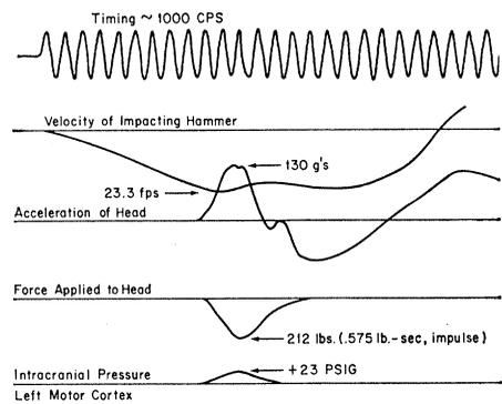
Fig. 1. Oscillographic record of physical measurements during impact; traces for velocity, acceleration, force, and intracranial pressure with a 1000-cy/sec time trace are displayed.
