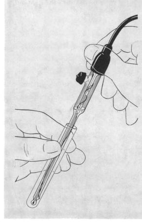
Consisting of a glass electrode and a silversilver chloride reference electrode sealed into a single body. Bulb wall thickness and strength provide a sturdier electrode than heretofore available. Electrodes are 6 inches long. Upper section is ½-inch diameter for use in standard electrode holders. Stem is ¼-inch diameter over the lower 4-inch length.
