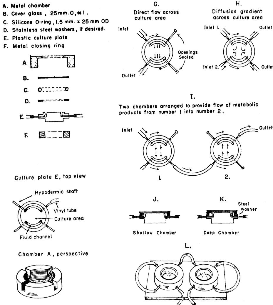
Fig. 1. Assembly of a microperfusion chamber. Details in the text.
