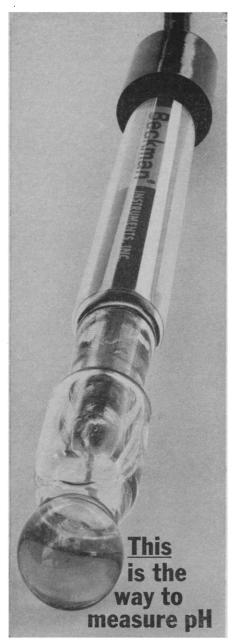
It's called the new Beckman E-3 Glass Electrode. It provides multi-purpose pH measurement. It offers wide temperature application in the 0-100° C range. It measures accurately over the entire 0 to 14 pH scale with low sodium error. It maintains high sensitivity to the sample in the presence of corrosive action.
