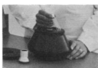
The Type 65 Fixed Angle Rotor. 65,000 rpm. 368,000 g.
