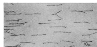
500X photomicrograph of uranium ions accelerated by MP Tandem striking photographic emulsion plate at 10 degree incidence. Note frequent collisions with atomic nuclei in emulsion.
