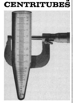
These polycarbonate graduated tubes are ideal for clinical work requiring precise graduations. Molded under extremely close tolerances, the accuracy of these graduations is well within Federal Specification Volumetric Apparatus, Glass-DD-581a.
