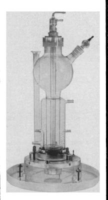
**Buchler Preparative Polyacrylamide Zone** Electrophoresis **Apparatus** (Poly-Prep)\*
