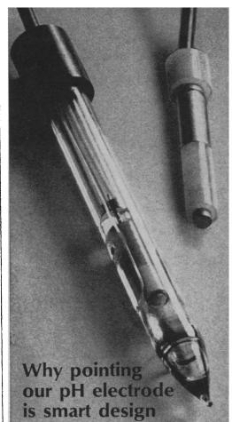
This new L&N glass electrode has been dropped on its tip 25,000 timesjust as it might if you let it fall into a beaker. It still works with full accuracy and sensitivity. No breakage. We've strengthened it at a critical point, where most electrodes are fragile.
