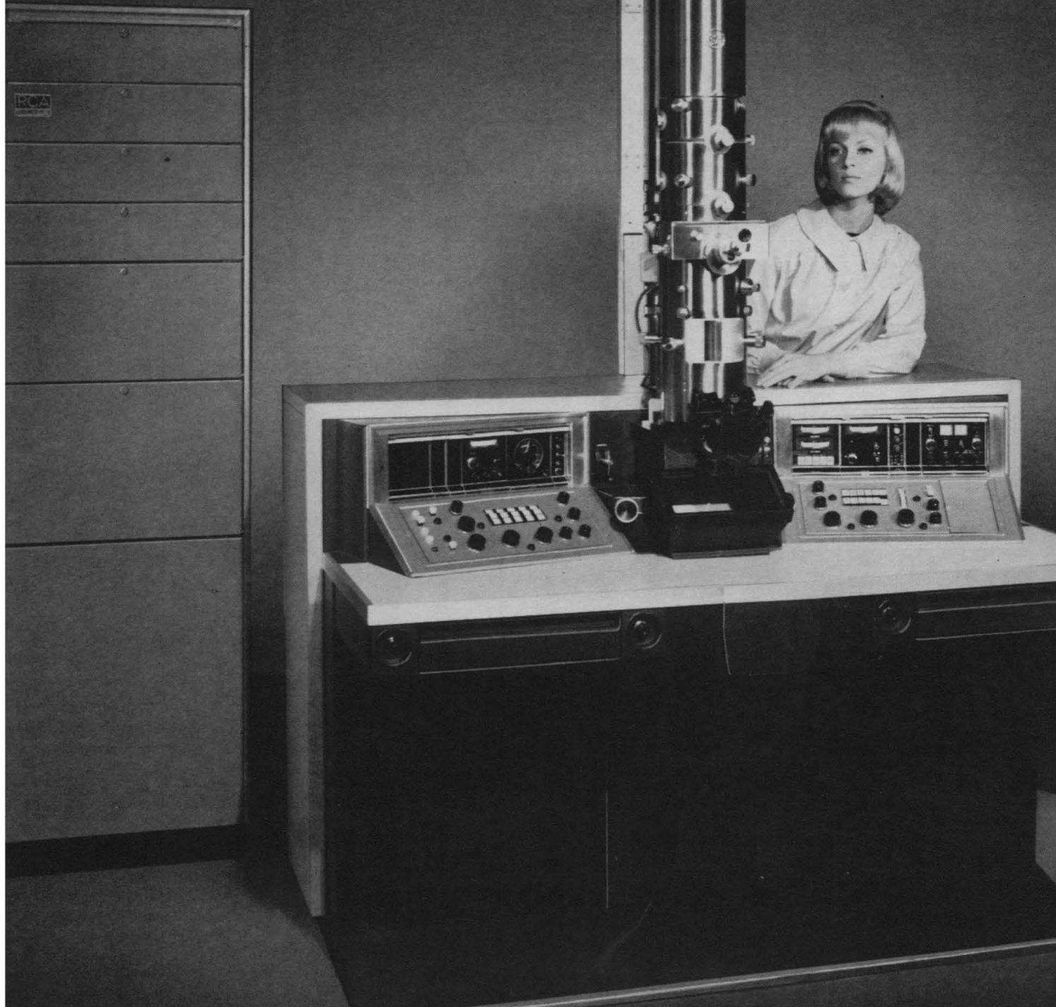
Complete EMU-4 Electron Microscope System. Includes television image intensification. Rack at left stores the mechanical fore pump and power supplies.
