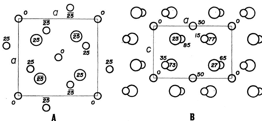
Fig. 1. (*A* and *B*) The structure of  $\text{Cu}_3\text{Se}_2$  projected on (001) and (100), respectively. Large circles represent Se atoms and small circles Cu atoms. Numbers give  $z$ -parameters in *A*, and  $x$ -parameters in *B*.
