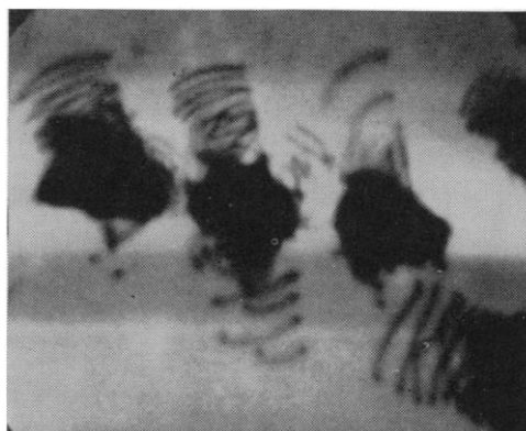
Large dark areas are regions of crystal damage caused by mechanical indentations in surface of silicon. Heat treatment relieved strain and caused edge dislocations, seen here as radiating lines or arc segments, to move outward from strained region. (800X magnification.)
