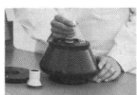
The Type 65 Fixed Angle Rotor. 65,000 rpm. 368,000 g.
