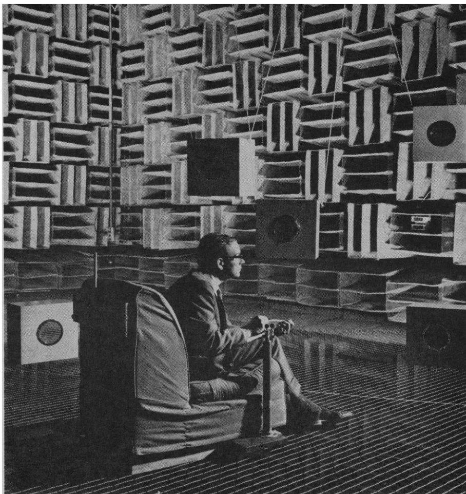
Fig. 1. Simulation of auditorium acoustics in an anechoic chamber ("free space" room). Speech and music signals are processed in a digital computer and radiated from suspended loudspeakers to create sound fields resembling those of actual auditoriums.
