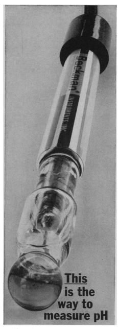
It's called the new Beckman E-3 Glass Electrode. It provides multi-purpose pH measurement. It offers wide temperature application in the 0-100° C range. It measures accurately over the entire 0 to 14 pH scale with low sodium error. It maintains high sensitivity to the sample in the presence of corrosive action.
