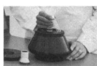
The Type 65 Fixed Angle Rotor. 65,000 rpm. 368,000 g.
