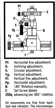
lash and vibration. The micromanipulator can conveniently be used for any motion by using vertical, horizontal, inclining and circular arc adjustments. The unit is supplied in a wooden case.
