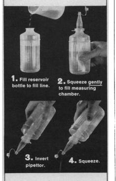
Use several for procedures requiring repeated dispensing of different reagents. Unbreakable ... resists most chemicals. Disassembles in seconds for cleaning and refilling. All units have 8-oz. polyethylene reservoir bottle with choice of 1, 2, 3, or 5 ml polypropylene measuring chamber. Price, \$4.50 each. May be assorted with other Nalgene Labware for maximum discount. Ask your lab supply dealer, or write Dept. 21261, The Nalge Co., Inc., 75 Panorama Creek Drive, Rochester, New York 14625.
