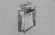
ELECTROPHORESIS TANK has "seethrough" Lucite walls that permit observation of entire run. Lightweight rack is adjustable for paper lengths up to 46". Ideal for separation of a wide variety of compounds, fingerprinting of peptides, amino acid mapping, preparative separations.
