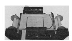
OSCILLOGRAM AMPLITUDE TABULATOR — Semi-automatic tabulating system for translating graphic records into printed tape output in 4-digit amplitude readings at 100, 256, or 1000 counts per inch. Scaling with a calibration curve eliminates further mathematical computation. Both linear and nonlinear records may be read from multi-channel recordings.
