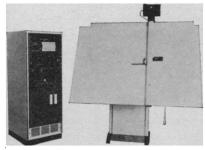
LARGE AREA COORDINATE DIGITIZER — For digitizing maps, graphs, layouts, drawings, or other graphic coordinate data for computer input. Also converts rough sketches into digital data for direct input to automatic artwork generators. Working surface is 48" square; resolution, 1000 counts per inch; accuracy, ±.005" over entire reading surface. Manual controls allow data insertion. Programmable output to punched tape cards, or typewriter.
