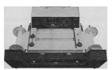
DIGITAL DATA READER — Reduces almost any X-Y recorded graphic data to digital form at over 10,000 tabulations per day. Output to punched cards, punched tape, or typewriter. A channel counter and time line counter are included. Input flexibility offered with keyboard for insertion of additional data by operator.
