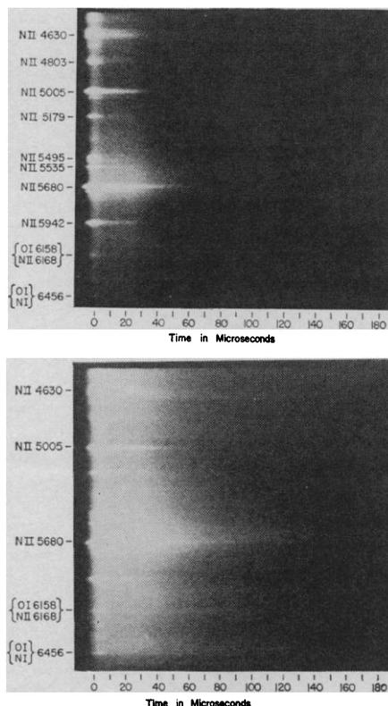
Fig. 1 (top). Time-resolved spectral components of a lightning stroke. Intense, unresolved multiplets are identified by the strongest line in the multiplet. Fig. 2 (bottom). The same negative used in Fig. 1 has been printed with less exposure to show the persistence of several lines for approximately 150  $\mu\text{sec}$ .
