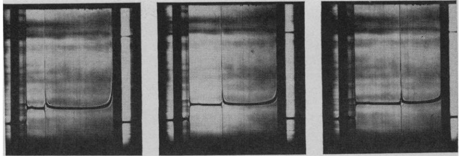
Fig. 1. Sedimentation patterns of myosin in 0.08M KCl, tris buffer 0.025M, pH 8.0. Protein concentration was 2.4 mg/ml. Examples of photographs (from left to right) taken at 6, 12, and 18 minutes after maximum speed of 59,780 rev/min was reached. The temperature was  $21^{\circ}\text{C}$ . The sedimentation coefficient of the peak is 21S and that of the minor one is 6.8S (corrected to  $20^{\circ}\text{C}$ ).
