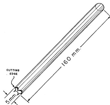
Fig. 1. Core-cutting sampling tube for NMR spectroscopy.
