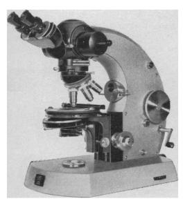
ZEISS Photomicroscope. This is the only microscope that has a built-in fully-automatic 35mm photomicrography system. The touch of a button determines exposure time, opens and closes the shutter, actuates the film counter, advances the film and resets the shutter for the next exposure. Complete interchangeability of all components and lighting systems extends this instrument's versatility to the maximum.
