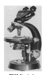
ZEISS Standard Microscope GFL. A larger, more rugged instrument, the GFL has all the features of the KF plus added capabilities for advanced studies. Interchangeable nosepieces allow for vertical or transmitted Illumination. A centerable condenser carrier permits use of Koehler illumination. The instrument features a separate coaxial coarse- and fine-focusing mechanism, and built-in illumination. The GFL can also be fitted with a great variety of stages.
