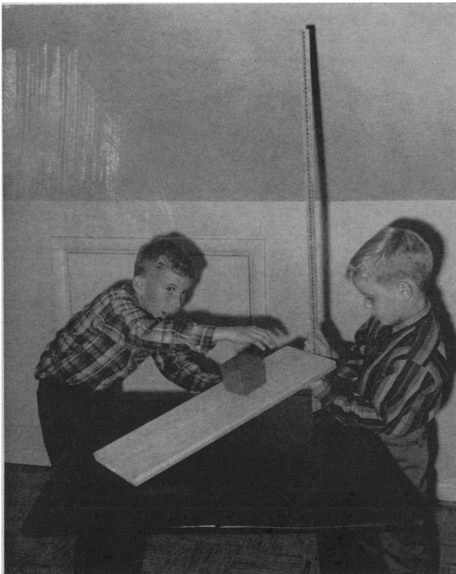
(Left top) An exercise dealing with the determination of smoothness in terms of resistance to sliding.
