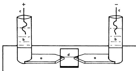
Fig. 1. Electrophoretic chamber. (a) Agarose bridges; (b) buffer reservoirs; (c) platinum wire electrodes; (d) polyacrylamide fiber on collodion-coated coverslip.
