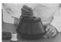
The Type 65 Fixed Angle Rotor. 65,000 rpm. 368,000 g.
