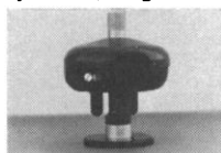
The SW65 Swinging Bucket Rotor. 65,000 rpm. 420,000 g.
