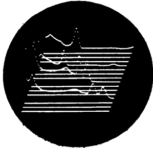
16 x 100-CHANNEL FORMAT—four separate detector inputs.
