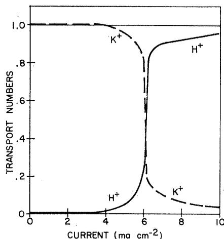
Fig. 1. Transport number of potassium and hydrogen ions across a cation-exchange membrane separating 0.005M potassium chloride solutions, when the system was well stirred, to produce a boundary-layer thickness of 30.1  $\mu$  (1).
