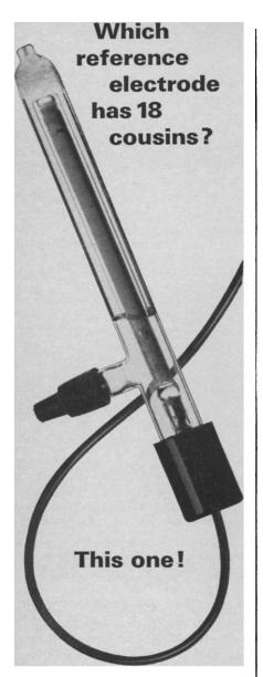
There are nineteen members in the family of Beckman Reference Electrodes-just so you can select the one best related to your requirements. There are four different types of reference junctions to pick from-asbestos fibre, palladium wire, ground glass sleeve, and porous frit. Each can be properly matched to your specific application for highly reliable determinations.
