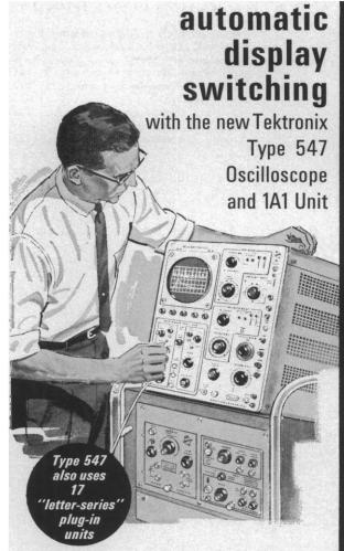
With Automatic Display Switching, the Type 547 provides two independent oscilloscope systems in one cabinet, time-sharing a single-beam crt.
