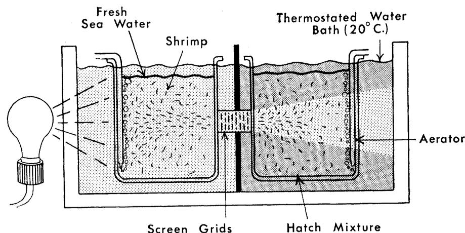
Fig. 1. Apparatus for separating active from inactive shrimp and from refuse.
