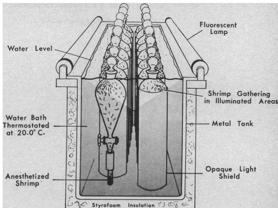
Fig. 2. Arrangement of the 16 separatory funnels as anesthesia chambers.
