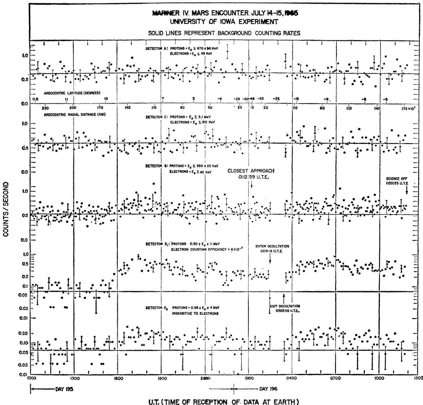
Fig. 2. A comprehensive plot of the counting rates of detectors A, C, B, D<sub>1</sub>, and D<sub>2</sub> before, during, and after the encounter with Mars on 14-15 July 1965. Note scale of positional coordinates of the spacecraft in upper part of the figure.
