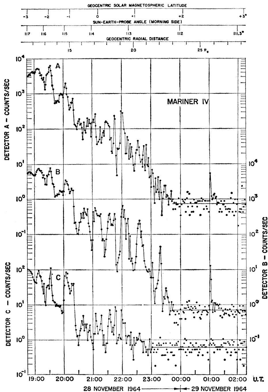
Fig. 1. Counting rates of detectors A, B, and C on Mariner IV during outward traversal of earth's magnetosphere.
